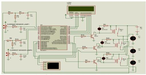
Figure 5. Simulation diagram of smart city lighting
