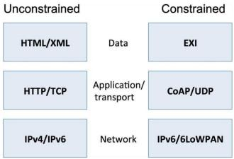
Figure 2. Protocol stack for IOT nodes
