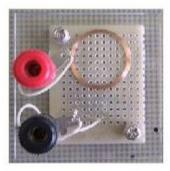
Figure 4. Coin type RFID tag
