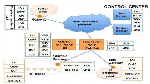
Figure 1. Components of IOT system
