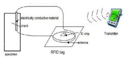
Figure 3. Outline of crack detection system
